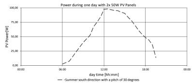
Equipped with two 50W panels it is possible to produce electricity to drive your TV set for more than 5 hours or to drive 13W energy saving bulb for more than 15hours.
